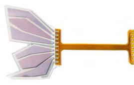
Size: OLED only (one wing): 50 × 35 mm<sup>2</sup> OLED w/ PCB: 50 × 85 mm<sup>2</sup>
