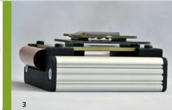
1 720p OLED microdisplay evaluation kit and driving electronics
