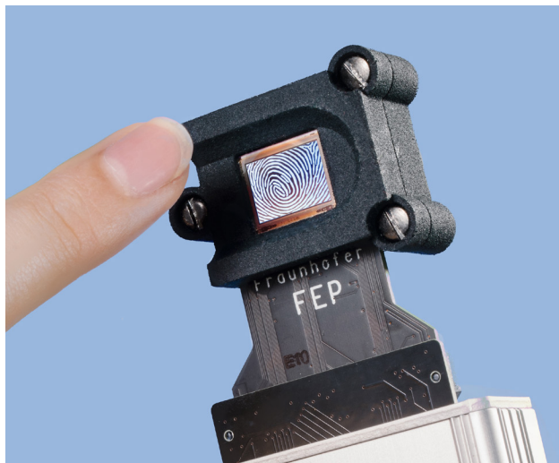
Fingerprint sensors based on bidirectional display technology
